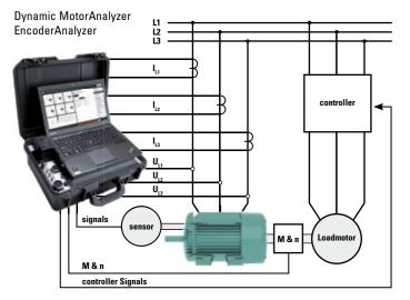
With the Dynamic MotorAnalyzer the user is also able to perform measurements at a load test rig. Torque-/speed characteristics can be determined with the Dynamic MotorAnalyzer, which is equipped with additional measuring inputs. Via these inputs, by using a torque measuring shaft, the torque and the speed signal as well as the temperature can be captured. In combination with the electrical input parameters, the system reliably delivers all information about the motor.
