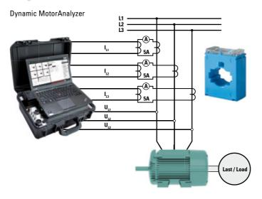
The motor to be tested is connected to the motor lead by means of voltage measurement connections and current clamps.
