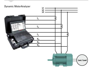
Measurement at motors with current transformer
