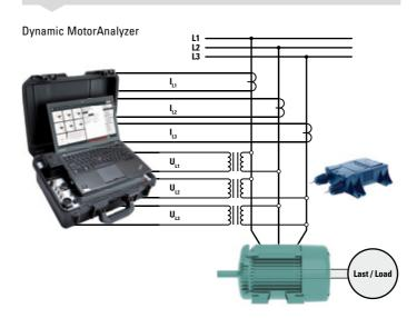
Voltage measurements in electric motors with high operational voltages are often performed with the help of voltage transformers. Here the Dynamic MotorAnalyzer is able to measure the voltage on the voltage transformer's secondary side. For this, only the transformation ratio and the type of transformer have to be entered. Afterwards the software re-calculates the measured values accordingly.
