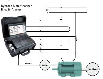
By combining the Dynamic MotorAnalyzer with the EncoderAnalyzer, SCHLEICH has developed a highly innovative instrument. This combination offers a great deal of value to the maintenance professional in performing dynamic monitoring and the comparison of various rotary encoder systems.
